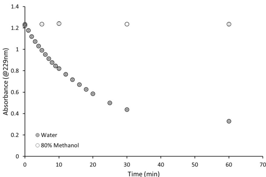
**Figure 15:** Spectrophotometric analysis of sinigrin hydrolysis kinetics in water and 80% methanol (n=3) by purified myrosinase (0.05 mg/ml) at room temperature (25°C).
