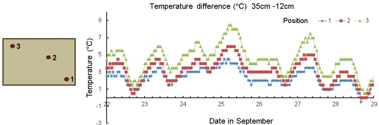
**Figure 39:** Temperature difference between 12 cm and 35 cm soil depth in a raised bed with under-soil heating set to maintain 18 °C. The three lines on the graph represent hourly data recorded in the three different positions of the bed as indicated on the schematic diagram on the left.
