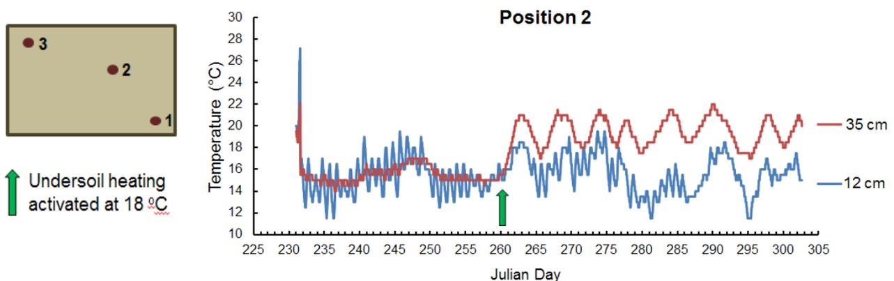
**Figure 38:** Hourly temperature recorded at 12 cm and 35 cm soil depth in a raised bed with under-soil heating set to maintain 18 °C from Julian Day 260 (indicated with green arrow). The data was recorded in Position 2 of the bed as indicated on the schematic diagram on the left.
