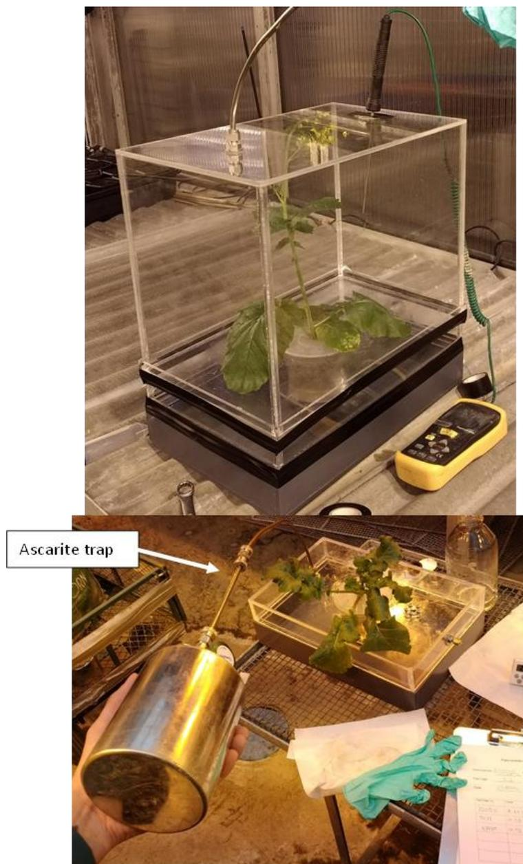
**Figure 45:** Plant volatile sampling chamber. The sampling chamber is depicted in use: **Top**, the assembled sampling chamber set up to sample volatiles from the aboveground biomass of the plant; **Bottom**, sampling volatiles from the belowground biomass, with the canister and Ascarite trap in place. The hole through which the roots of the plant are separated from
